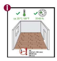
Please note that typical living room temperatures must prevail throughout the year (VOB, Part C, DIN 18365, DIN EN1264, DIN 4725). The room air temperature should be approx. 20°C, the relative humidity should be between 35-60%.
